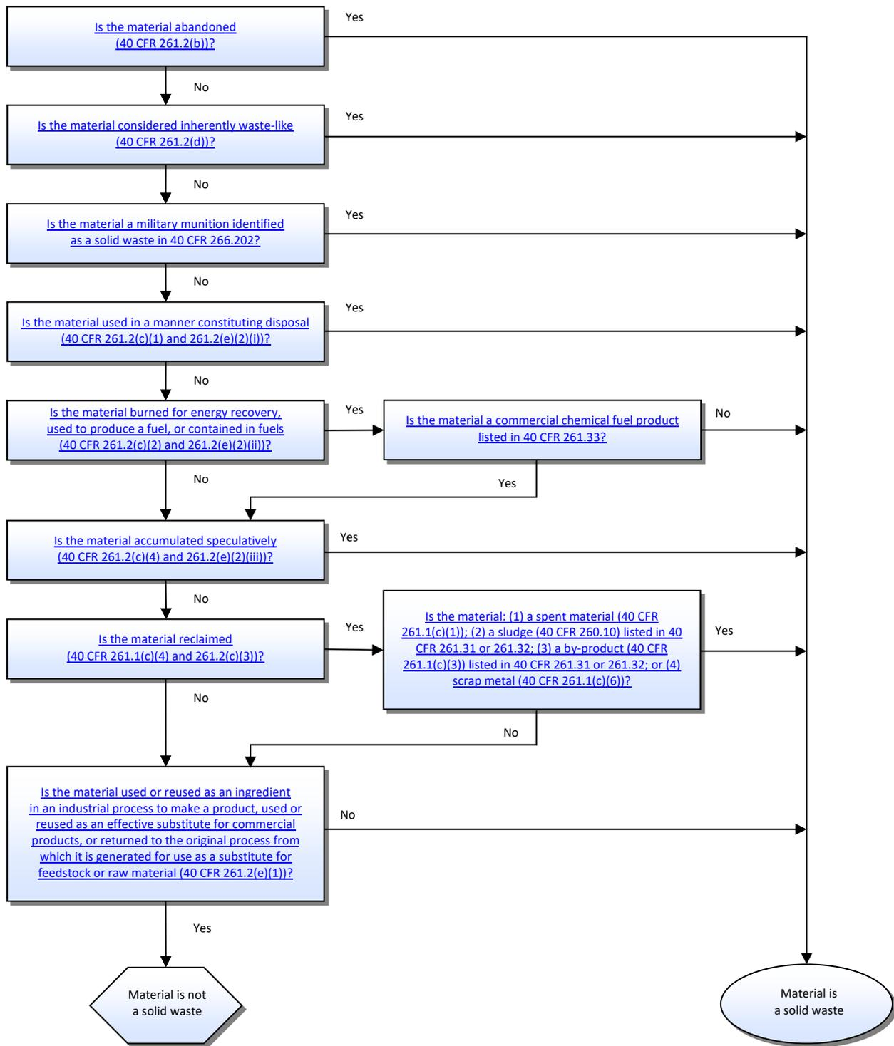
Exhibit 1-1. Determination Flowchart “Is the Material a Solid Waste?”
