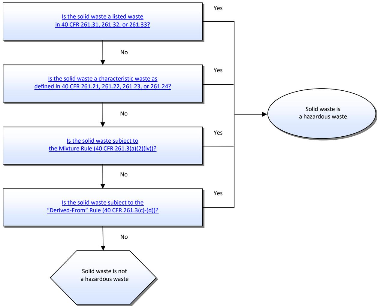
**Exhibit 1-3.** Determination Flowchart “Is the Solid Waste a Hazardous Waste?”
