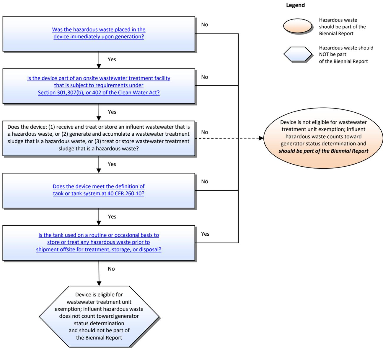
**Exhibit 2-1.** Determination Flowchart for Hazardous Wastewater Reporting “Was the Waste Managed in a Device Eligible for the Wastewater Treatment Unit Exemption?”
